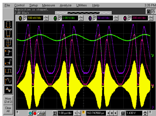
Figure 4: Oscilloscope traces of 380kHz drive signal (green), corresponding to 760kHz A-scan. Shown are laser output (red), amplified output (purple) and Mach-Zehnder clock fringes (yellow). Note nearly symmetric forward/backward scans.
