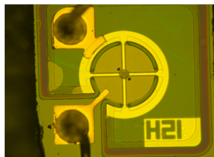
Figure 1: Device cross section (left) and top-view wire-bonded photo (right). Device employs an InP-based MQW gain region, a wafer bonded fully oxidized AlGaAs mirror, and a suspended dielectric mirror above a variable air-gap. Device is optically pumped from the top at 980 nm, and emits 1310 nm laser light out the same side.
