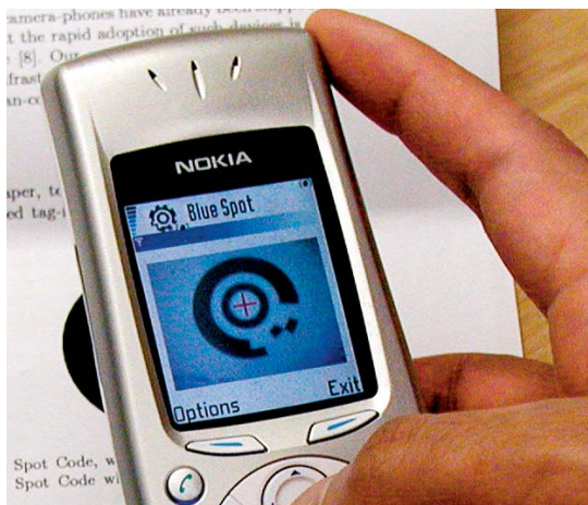
Circular symbols turn a camera phone into a wireless mouse.
