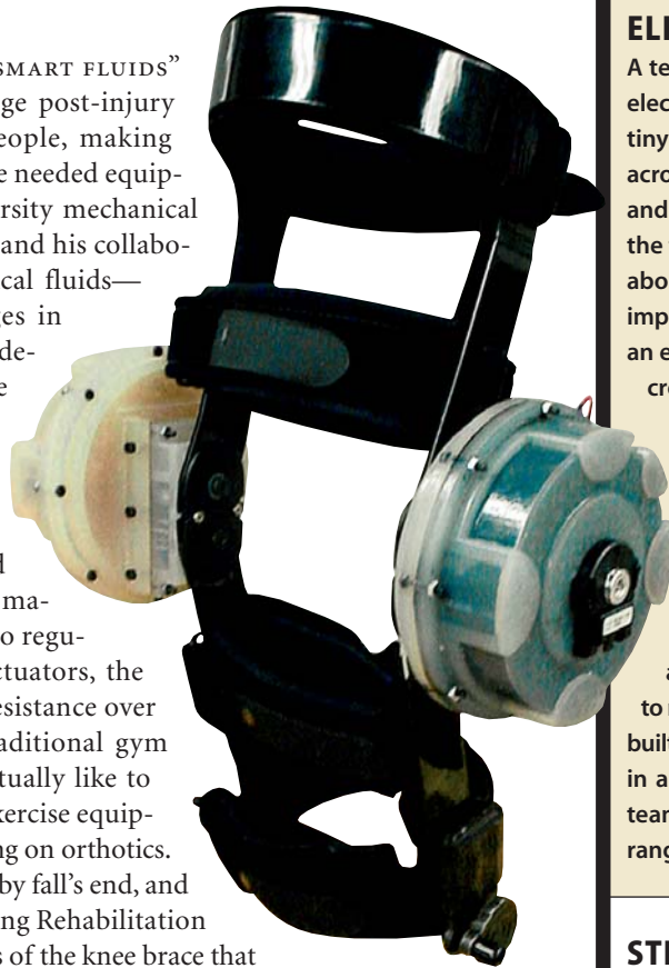
“Smart fluids” control this brace.
